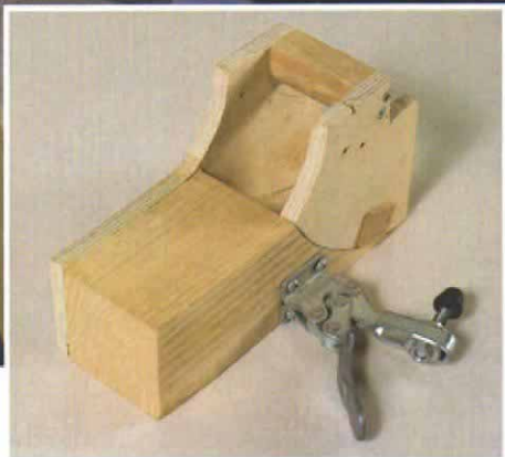
Shop-made jig makes cutting odd-shaped fittings an easier and safer task. Fixed to the saw table by a bar clamp, the jig secures the fitting at the desired angle. Adjustment can be made by loosening the toggle clamp.
