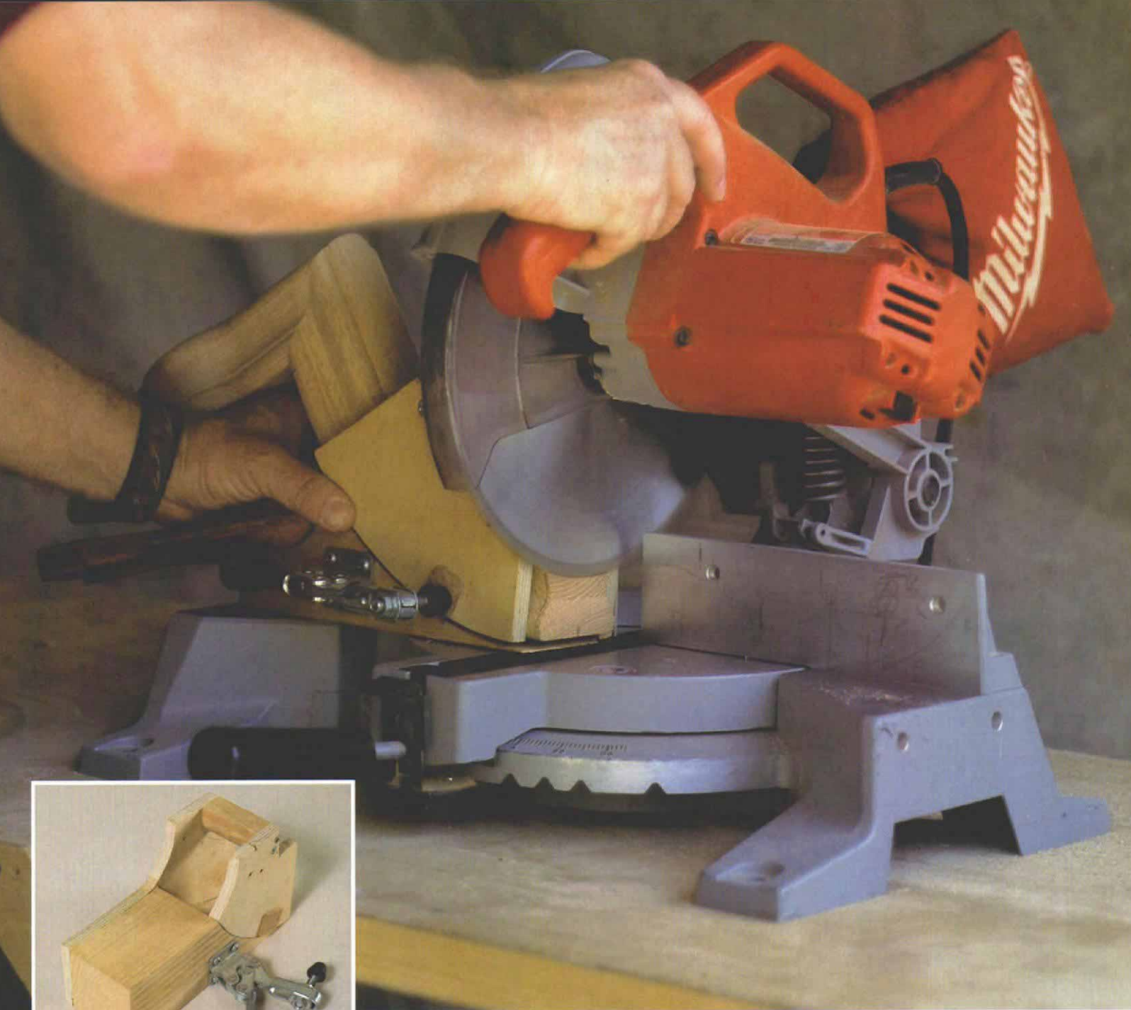
Shop-made jig makes cutting odd-shaped fittings an easier and safer task. Fixed to the saw table by a bar clamp, the jig secures the fitting at the desired angle. Adjustment can be made by loosening the toggle clamp.
